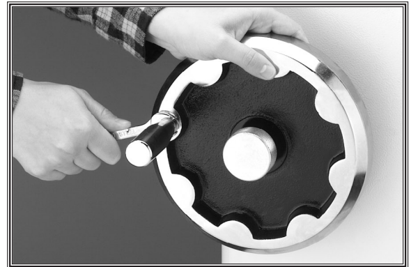
Figure 22. Installing handwheel, lock knob and handle.
